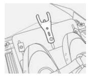
The removable bracket, with suction cups on it, is for use in boats that you row only occasionally and it is attached by wetting the cups and pressing them down onto a flat surface (normally on the stern of the boat). The bracket is hinged so that you can adjust it to the optimum viewing angle. On some boats the suction cups will hold on less well than on others so be aware of this and make sure you attach the lanyard to the boat.
