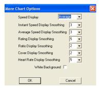
'Speed Display' enables either, 'instant', 'average' or 'both' to be charted. The 'instant' shows the speed every approx 20mS. This will show the velocity profile through the stroke. The 'average' is the average speed for the stroke and 'Both' displays both 'instant' and 'average' speeds. Note: If record has been recorded in Macro mode, then Speed Display should be set to average.
