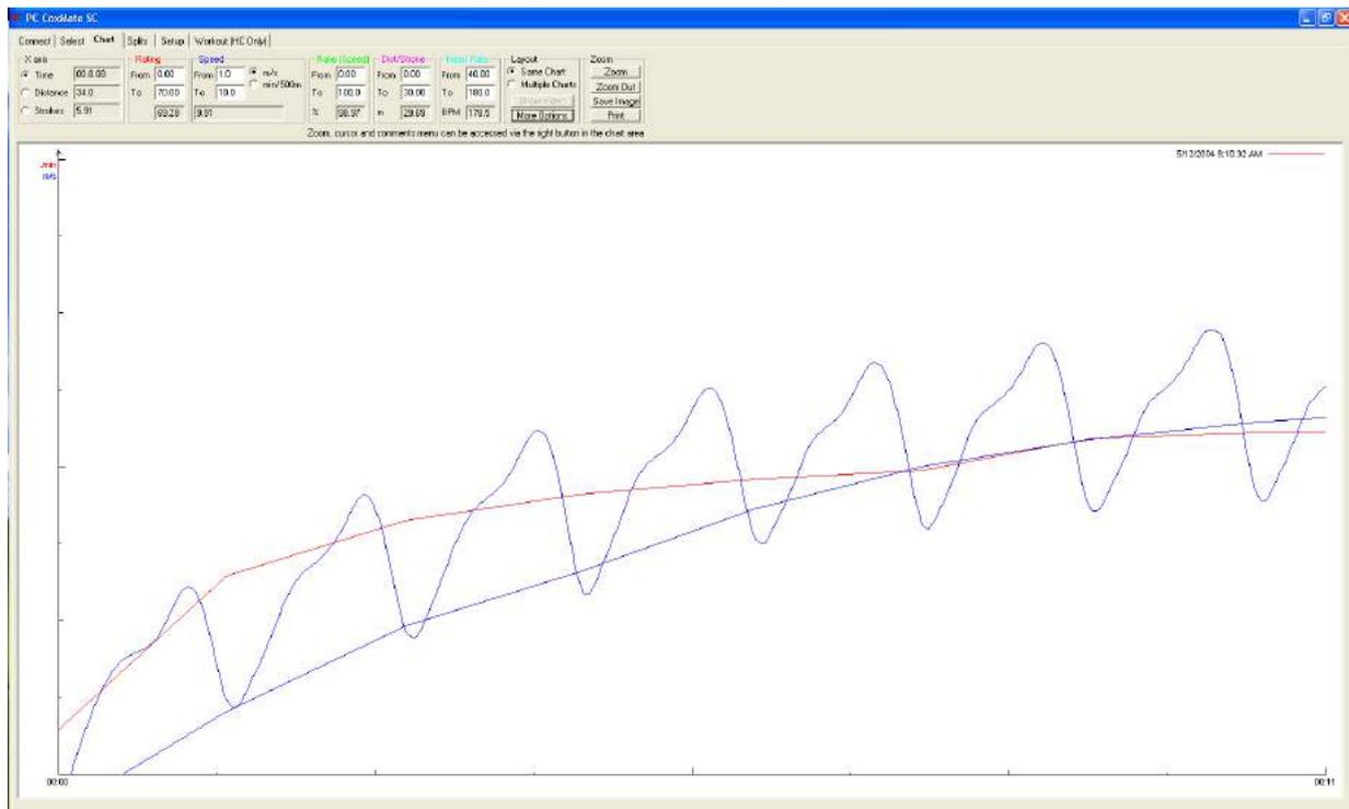
The above graph shows the first 7 strokes of a start. The blue lines show both instantaneous speed and average speed (averaged over a stroke speed). The instantaneous speed shows how the boat speeds up and slows down through the stroke.
