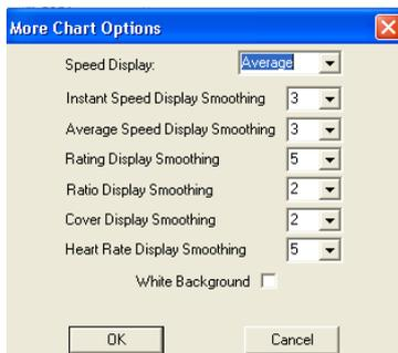
'**Speed Display**' enables either, '**instant**', '**average**' or '**both**' to be charted. The '**instant**' shows the speed every approx 20mS. This will show the velocity profile through the stroke. The '**average**' is the average speed for the stroke and '**Both**' displays both '**instant**' and '**average**' speeds. Note: If record has been recorded in Macro mode, then Speed Display should be set to average.
