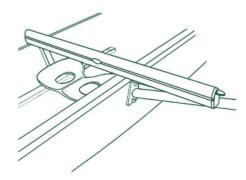
② Gently pull the tool towards you so that the fixed end stop is in contact with the far side of the boat.
