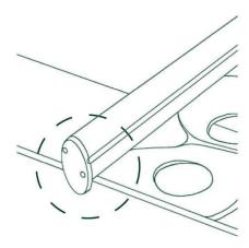
(3) Slide the moving stop up against the near side of the boat and hold it there with one hand.
