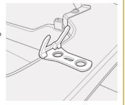
The suction cup bracket can also be used to mount the unit to a foot stretcher screw by removing the suckers.
