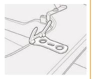
The suction cup bracket can also be used to mount the unit to a foot stretcher screw by removing the suckers.
