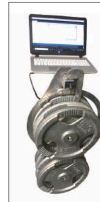
Static calibration rig, using weights measured to 1g accuracy.
