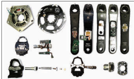
Cycling power meters, from all the major manufacturers, were taken apart.
